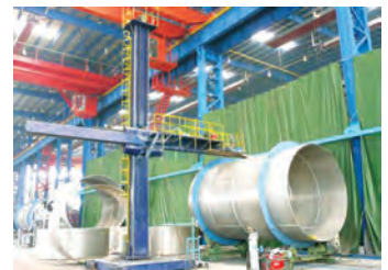
Outside Welding Machine
